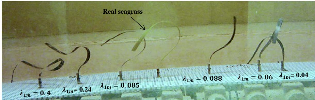
Figure 1. The behavior of model seagrass leaves with  $\lambda_{1,m} \approx 0.4$  to 0.04 in comparison with the real *P. australis* leaf. The model blade with  $\lambda_{1,m} = 0.085$  exhibits the most realistic motion.
