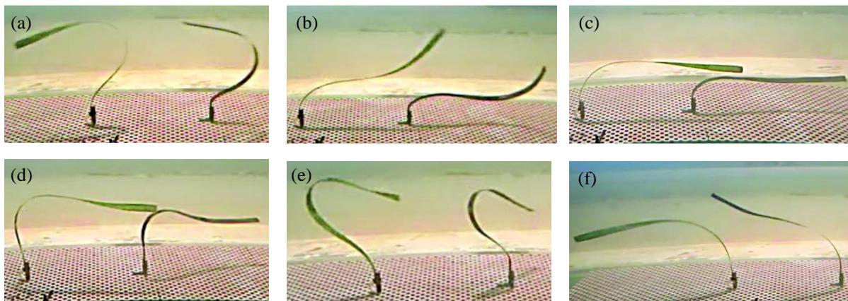
Figure 2. Comparison of the real and designed blades under different wave cycles. Figures 2a to 2c display the behaviour of the designed seagrass blade when the fluid motion is from left to right and Figures 2d to 2f display the blade motion when the fluid motion is from right to left. The real seagrass leaf is on the left hand side in all photos.
