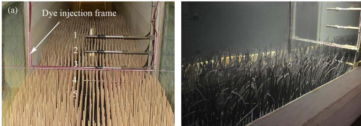
Figure 3. Photographs showing examples of (a) rigid and (b) flexible canopy as well as the dye injection setup was placed mid-length of the canopy in both cases.
