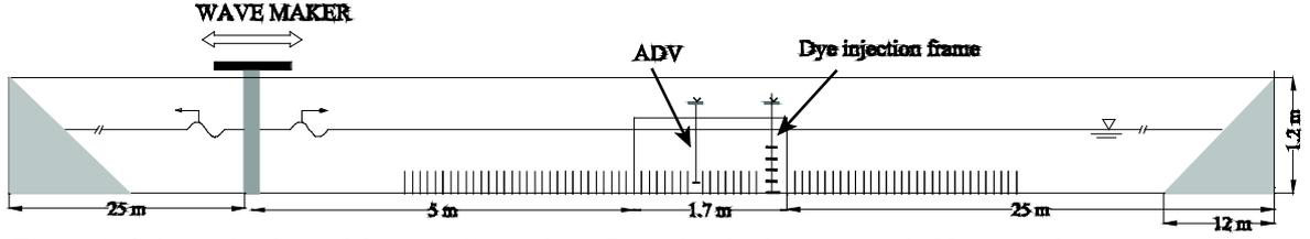
Figure 1. Schematic view of the experimental configuration in the wave tank. Not to scale.
