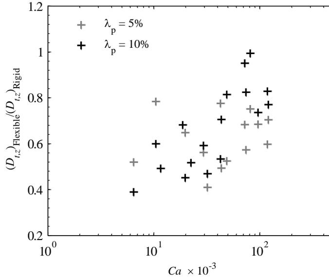
Figure 6. Flexible to rigid diffusivity values plotted against  $Ca$ . The  $(D_{t,z})_{Flexible} / (D_{t,z})_{Rigid}$  values, unexpectedly, increases by increasing  $Ca$ .
