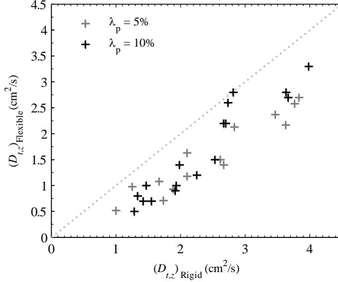
Figure 4. Values of vertical turbulent diffusivity,  $D_{t,z}$ , observed within a flexible canopy plotted against  $D_{t,z}$  observed within a rigid canopy.  $D_{t,z}$  values are almost always lower within a flexible vegetation.
