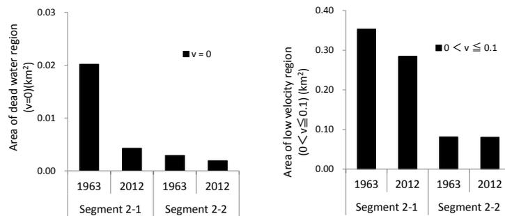
Figure 5. The histogram of area Left: dead water region Right: low-velocity area
